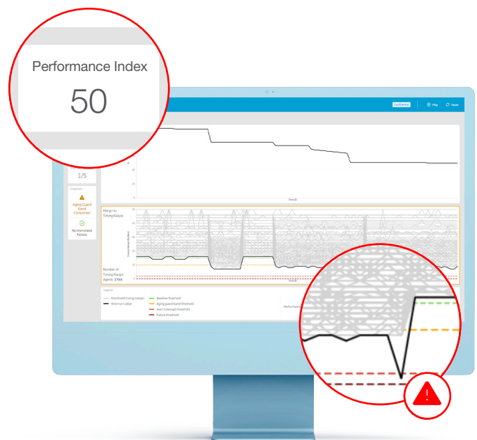
Figure 9: Visualization of RTHM in a 5nm chip: real-time indication of a severe margin drop in a device that might cause SDC.
